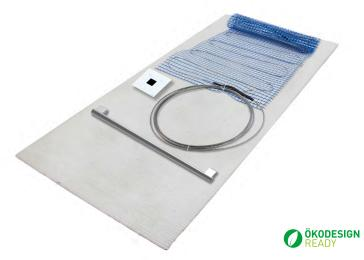
The flush-mounted ZESTO hand towel warmer is a wall heating set consisting of a heating mat and limiter (approx. 60 °C), an eTOUCH HYBRID designer fixed thermostat with its sophisticated look and smart button programming, a high-quality, chrome-plated KEUCO towel rail, and an insulating plate.
